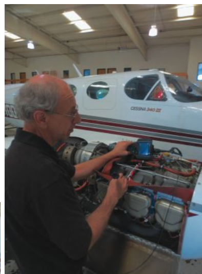
Scott Utz of Arapahoe Aero uses his shop's GE XL VU videoscope to examine the engine of a Cessna 340, left. Using the articulating camera head, a healthy exhaust valve can be seen clearly, below.
