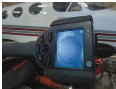
Scott Utz of Arapahoe Aero uses his shop's GE XL VU videoscope to examine the engine of a Cessna 340, left. Using the articulating camera head, a healthy exhaust valve can be seen clearly, below.
